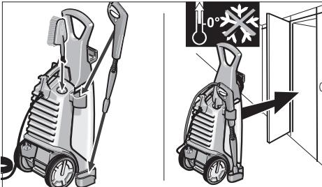
**Caution!** Frost can destroy an incompletely emptied unit. In the winter keep the unit in a frost-free room.
